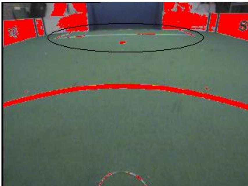
Figure 2.2: *Simple white line detector*. In a simple white line detector the pixels that meet the conditions for being white (thresholds on the red, green and blue values) are painted red to see if it detects the white (lines) the right way. As can be seen in this figure white lines that lie further away are too small and not defined as white lines. What is supposed to be seen as a solid line will be detected as a broken line.
