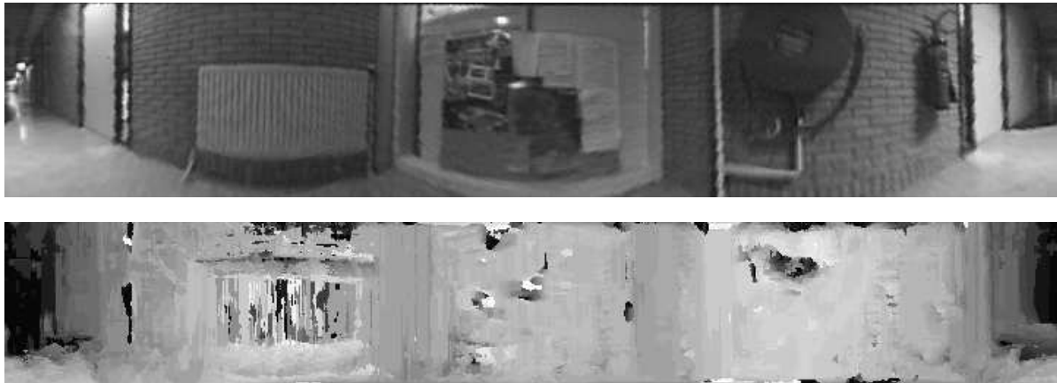
Figure 4.10: (top) The reference image. (bottom) The depth map computed from the reference image and 4 other images.
