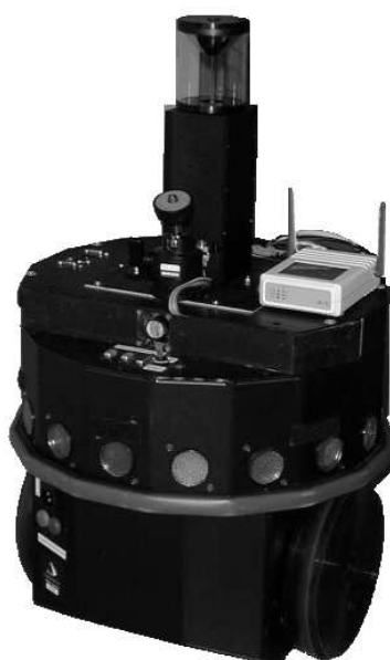
Figure 1.1: Our experimental platform. The robot is a Nomad Super Scout II, manufactured by Nomadic Technologies Inc. The panoramic vision sensor, manufactured by Accowle Inc., is situated on top of the robot.
