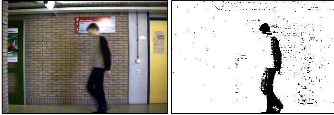
Figure 5.1: (Left) A frame from video sequence that presents a static scene and a person in motion. (Right) Results of segmentation based only on temporal cues for individual pixels. Note incorrect segmentation of image regions (torso) where the color of the background coincides with the object.
