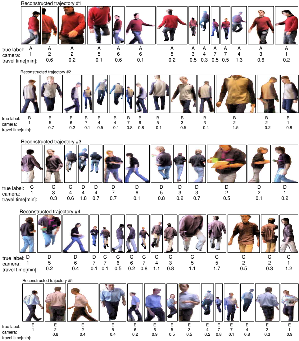
Figure 3.9: Trajectories defined by a partition \omega estimated by our algorithm. Every image represents a frame from a person’s pass through the field of view of some camera. The “true labels” indicate the ground-truth association. The numerical camera indicators correspond to Fig. 3.5. From the true labels, we see that the trajectories #1, #2, #5 were reconstructed correctly, the trajectories #3 and #4 are mixed.
