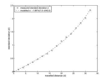
Figure 1: The standard deviation of the ball vs. the travelled distance.
