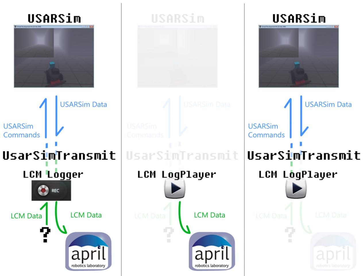
Figure 5: Demonstration of how the LCM logger and LogPlayer can be used. The left pane shows that the LCM logger captures all LCM messages. The middle pane shows how the LogPlayer can be used to simulate the session in a April module, and the right pane shows how the session can be simulate the session in USARSim.
