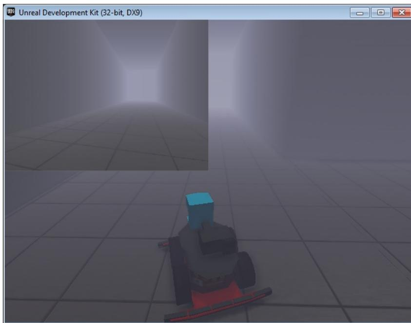
Figure 1: The `P3AT` agent spawned in USARSim environment, sending to LCM channel.
