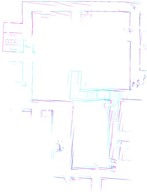
Figure 5.14: The result of Hough map stitching for experiment 3. Cyan parts are from piece 1, magenta are from piece 2. Blue parts show overlap from both pieces.
