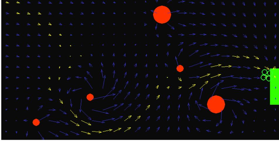
Figure 1: Potential Field, leading a drone towards a goal (simple simulation)
