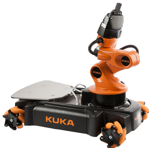
Figure 5: The KUKA youBot with the arm attached to the omnidirectional platform.
