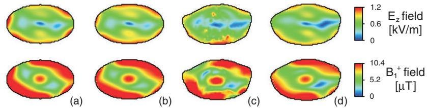
**Figure 6.** Comparison between FDTD and BBM results at 7 T for RF shimming. (a) Homogeneous ellipse, FDTD. (b) Homogeneous ellipse, BBM. (c) Segmented patient, FDTD. (d) Homogeneous patient, BBM.
