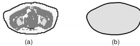
**Figure 2.** Difference between the female anatomy model for the FDTD method that has been segmented in (from light to dark) fat, bone, muscle and air (a) and the female anatomy model for the BBM method (b). Note that the contour of the BBM model is based on the contour of the FDTD model, but that the boundary has been smoothed to remove any staircasing that hampers the matching at the boundary.
