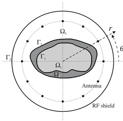
**Figure 1.** A two-dimensional model of the inside of a conventional MRI scanner that forms the calculation domain. Various regions ( $\Omega_1$ ,  $\Omega_2$  and  $\Omega_3$ ) and boundaries ( $\Gamma_1$ ,  $\Gamma_2$  and  $\Gamma_3$ ) are identified.
