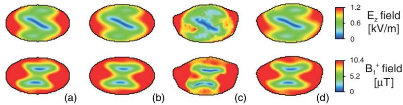
**Figure 4.** Comparison between FDTD and BBM at 7 T for quadrature settings. (a) Homogeneous ellipse, FDTD. (b) Homogeneous ellipse, BBM. (c) Segmented patient, FDTD. (d) Homogeneous patient, BBM.
