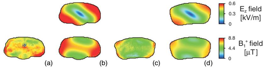
**Figure 5.** Comparison between measurements and BBM at 3 T for quadrature settings. (a) Real patient, measurement. (b) Homogeneous patient, BBM. (c) Real patient, measurement. (d) Homogeneous patient, BBM.
