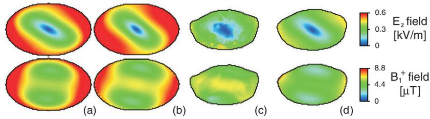
**Figure 3.** Comparison between FDTD and BBM at 3 T for quadrature settings. (a) Homogeneous ellipse, FDTD. (b) Homogeneous ellipse, BBM. (c) Segmented patient, FDTD. (d) Homogeneous patient, BBM.
