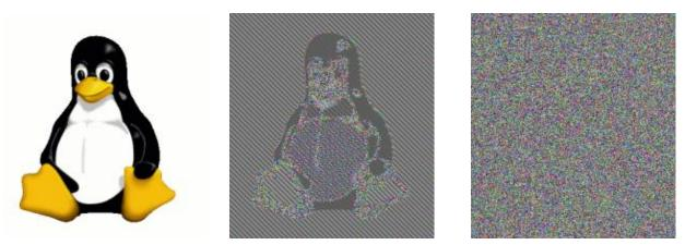
left: original picture, middle: encrypted using ECB mode, right: secure encryption mode Image credit: Larry Ewing, The GIMP, wikimedia.org.
