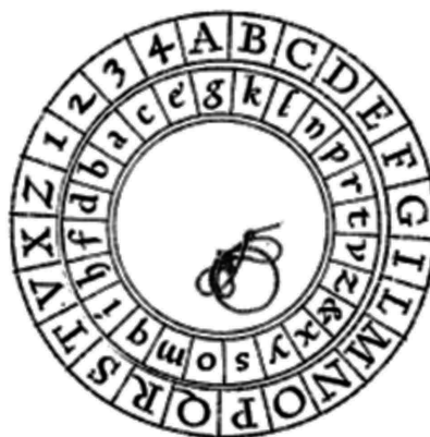
Figure 2.1: An example of an Alberti cipher disk in which the g is matched to an A.
