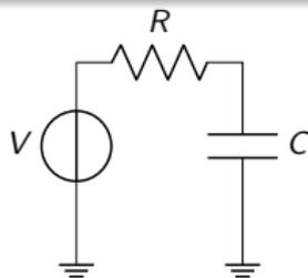
The voltage source  $V_V$  is considered exogenous; the resistance  $R$  and capacitance  $C$  are considered exogenous and static; the initial condition  $V_C(t_0)$  is considered exogenous.
