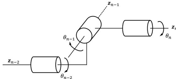
Figure 1: An example of a serial robot with an offset between the  $n - 2$  and  $n - 1$  joints.
