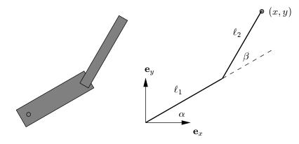
We control the robot by changing  $\alpha$  and  $\beta$ , but for a task we are interested in where the hand is.
