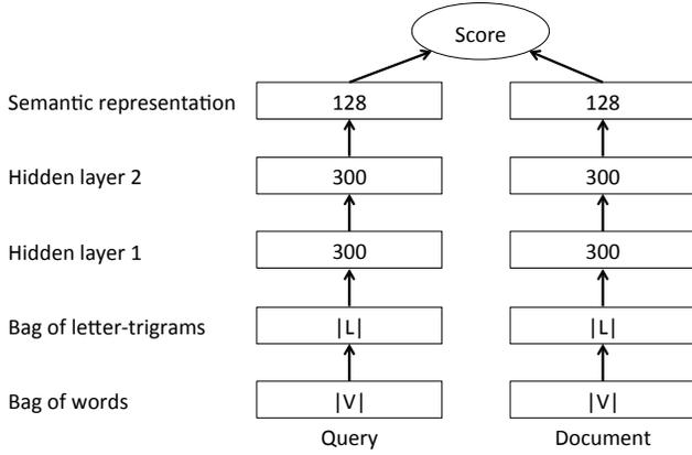
Figure 3: The Deep Structured Semantic Model (DSSM) [20].
