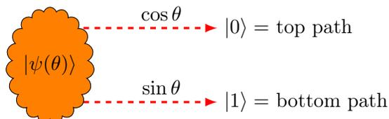
For example, the state  $|\psi(0)\rangle = |0\rangle$  represents a photon that is fully on the top path while  $|\psi(\pi/2)\rangle = |1\rangle$  corresponds to a photon fully on the bottom path. In general, a photon can take both paths simultaneously in superposition. This corresponds to a general state  $|\psi(\theta)\rangle$  in equation (3).
