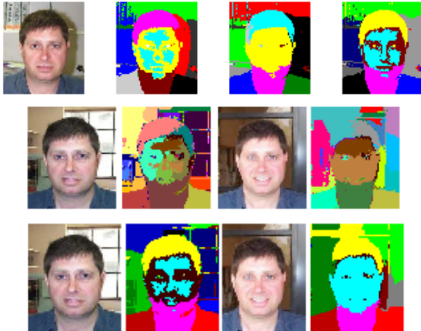
Figure 2. Top row: From left to right: an example segmentation produced by the baseline method, memory bounded algorithm with 30% of total images and 125 clumps, and the memory bounded algorithm with no images merged and 125 clumps. Row 2: Example clump distributions. Pixels of the same color are summarized in a single clump. Row 3: segmentations corresponding to clumps in row 2.
