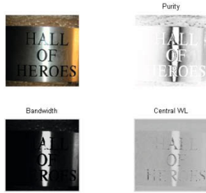
Fig. 9. Representation of \alpha , \delta and \lambda components computed for image (d) in Fig. 1
