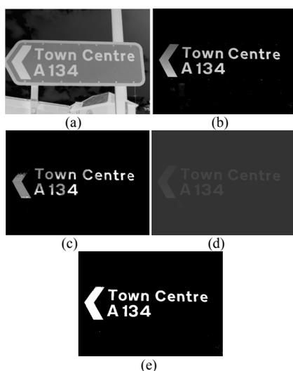
Figure 4. (a) The original Image (b) Gamma correction  $\gamma=2$  applied to connected opening enhanced image (c) Gamma correction  $\gamma=4$  applied to connected opening enhanced image (d) Difference between gamma corrected images (contrast enhanced by 20%) (e) Thresholded
