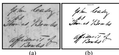
Figure 7. (a) Input Image with simple background (b) Threshold image (Significance level of 10% corresponds here to an intensity value of 137).
