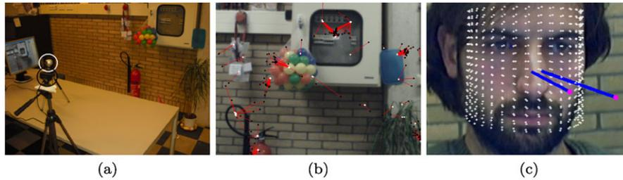
**Fig. 4** (a) The system setup consisting of a “subject camera” (white) and a “scene camera” (black); (b) the displacements (red) between the original location of the “head fixations” (black) and the adjusted
