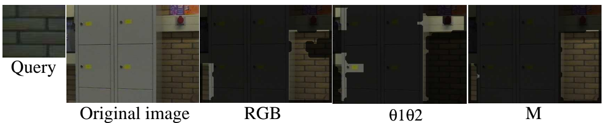
Fig. 4. a. Query texture under different illumination b. Target image c. Segmentation result based on \nabla C_{RGB} . d. Segmentation result based on \nabla C_{\theta_1\theta_2} . e. Segmentation result based on color ratio gradient \nabla C_M .
