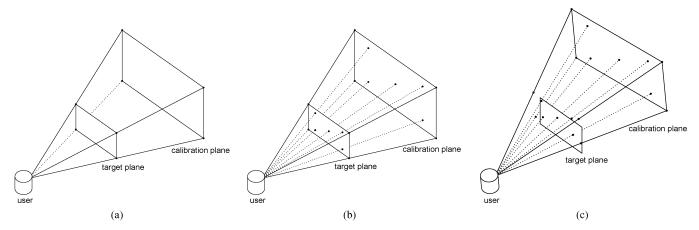
Fig. 10. (a) The construction of the calibration plane, (b) the intersection of the calibration points on known target plane points, and (c) the effect on the known points on the target plane while moving the head in the 3-D space.
